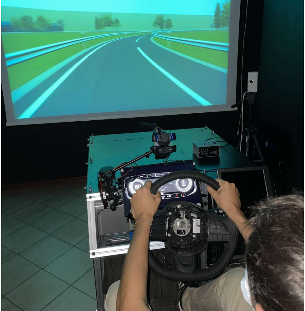
Figure 7.2: Real-Time System installed on simulator. Above the speedometer you can see the video camera and behind on the right you can see our module as a silver box with a black panel in front.
